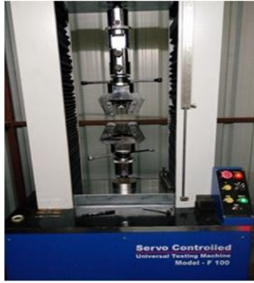
Figure 4.20 Servo controlled universal testing machine
