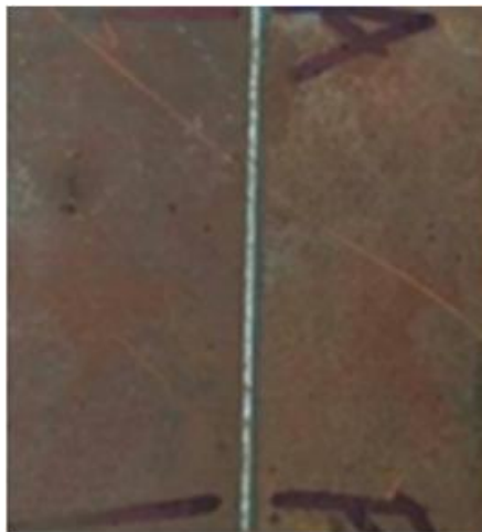
Figure 4.13 Laser weld on plate
