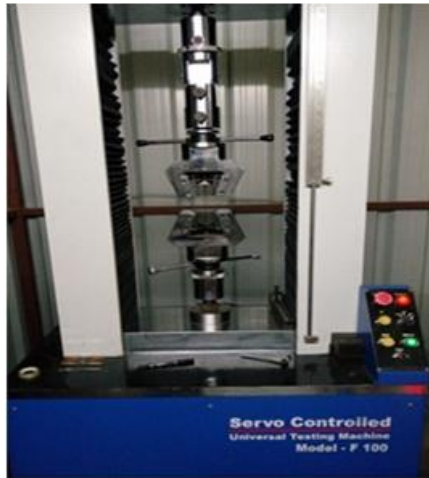
Figure 4.22 servo controlled universal testing machine
