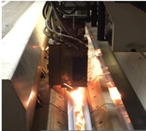
Figure 4.16 Balliu Belgium machine used for Laser cutting
