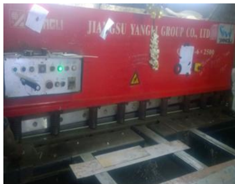
Figure 4.3 Hydraulic Shear Cutting of Corten A588 sheet
