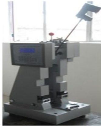
Figure 4.24 laryee Izod and charpy universal Impact tester
