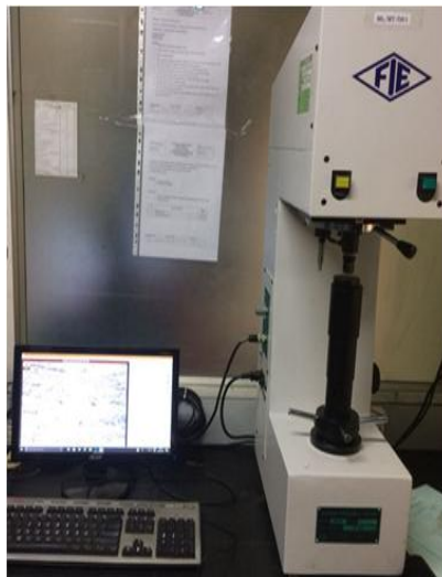
Figure 4.26 FIE Rockwell Hardness testing machine
