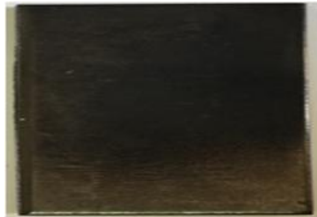
Figure 4.2 2mm Thick sheet Corten A588 plate before processing for welding
