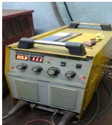
Figure 4.8 Pentagon tig 400 machine used for GTAW
