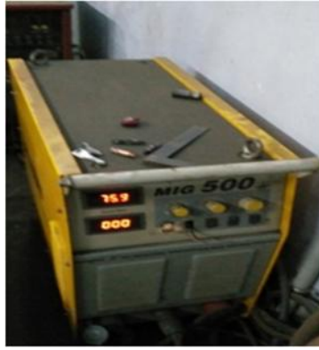
Figure 4.10 Pentagon mig 500 machine used for GMAW
