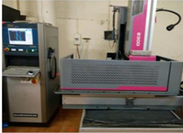
Figure 4.18 Cnc EDM wire cutting
