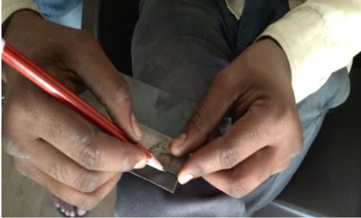
FIG 4.10 MARKING OF DIMENSIONS ON MOTOR SUPPORT PLATE
