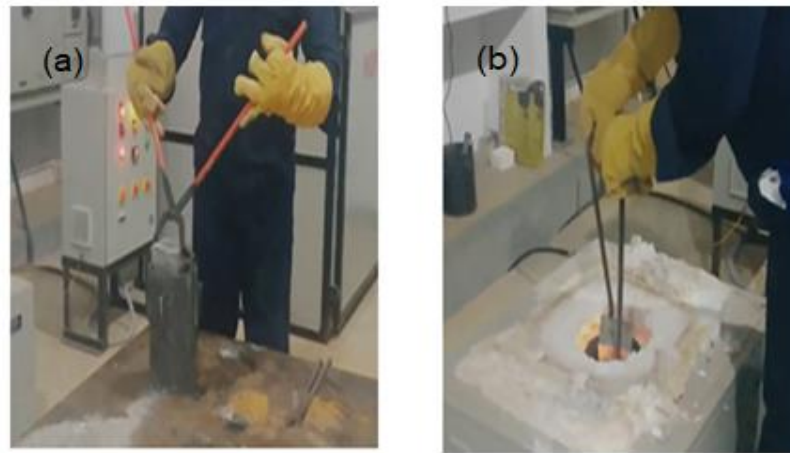
Fig. 4.5 (a) Placing pure magnesium in Stainless Steel Crucible and (b) Placing of stainless-steel crucible in the Electrical resistance furnace
