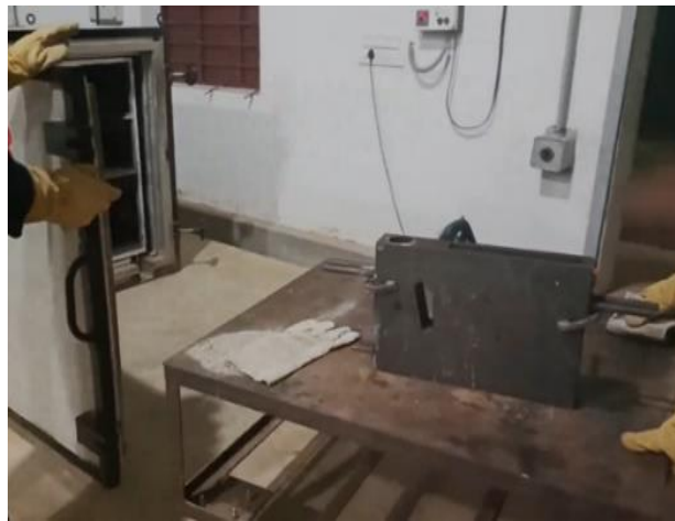
Fig. 4.4 Die cast steel mold about to be kept in the oven
