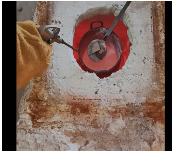
Fig. 4.7 Addition of Mg-Sr master alloy (or) gadolinium
