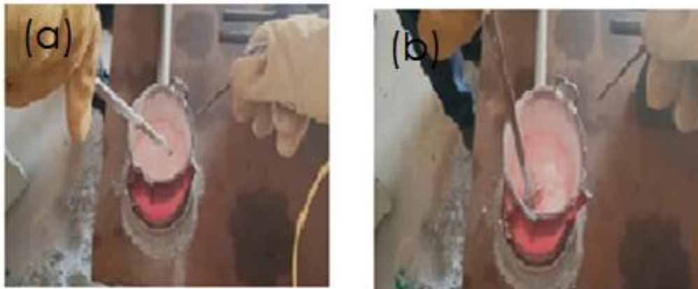
Fig. 4.9 (a) Hand stirring process and (b) Skimming process
