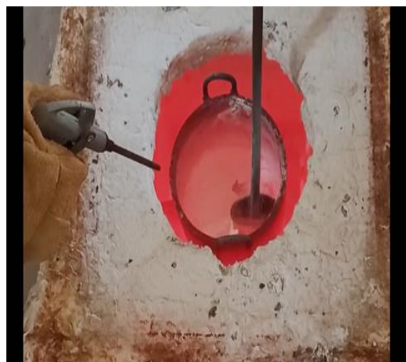
Fig. 4.6 Skimming under protective atmosphere
