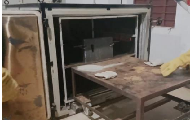
Fig. 4.8 Removal of preheated die cast steel mold from preheated oven
