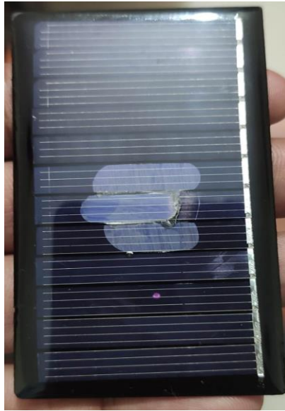
Fig 5.9:-Burned solar cell
