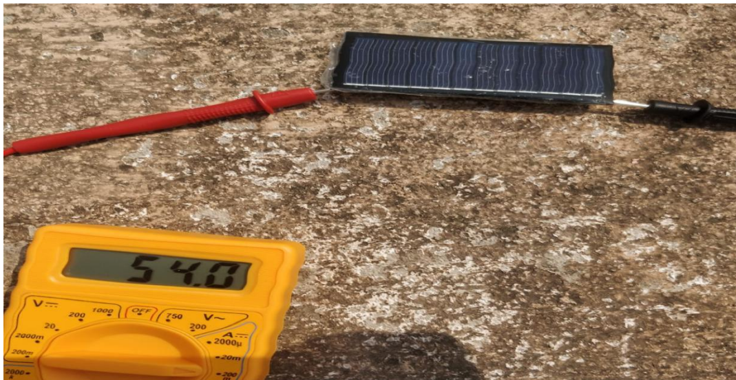
Fig4.1: Multi-meter with solar cell
