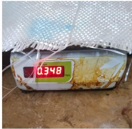
Fig 4.6: Weight of s-glass fibre
