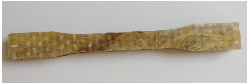
Fig 4.11: Tensile test specimen ASTM-D638
