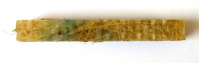
Fig 4.12: Flexural test specimen ASTM-D790
