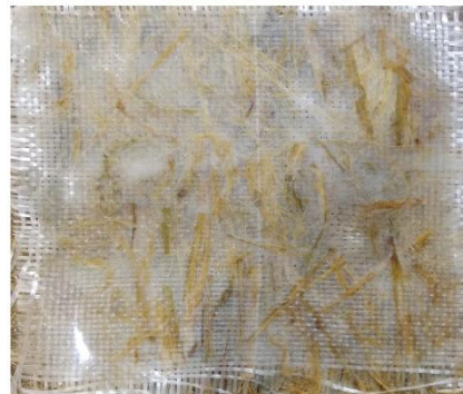
Fig 4.10: Finished plate after curing
