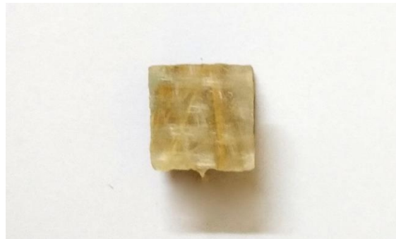
Fig 4.14: Hardness test specimen ASTM-D785
