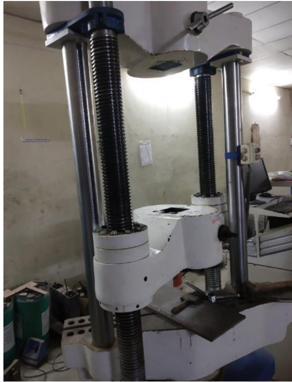
Fig 5.1 compression testing machine
