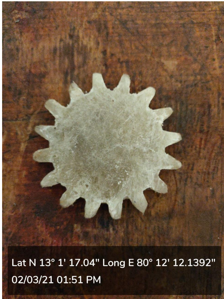
Fig 4.21 composite spur gear
