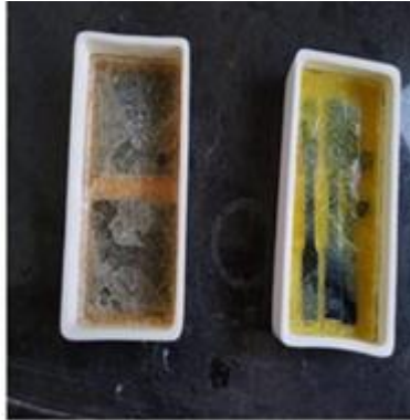
Fig:23 Inconel 625 Specimens after 25 hours of Heating
