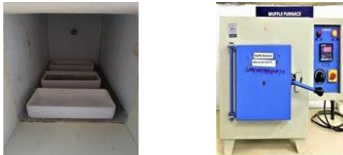
Fig:22 Alumina Crucibles in Muffle furnace and Heating process
