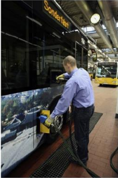
Fig.1.10: Urea is added to the exhaust gasses
