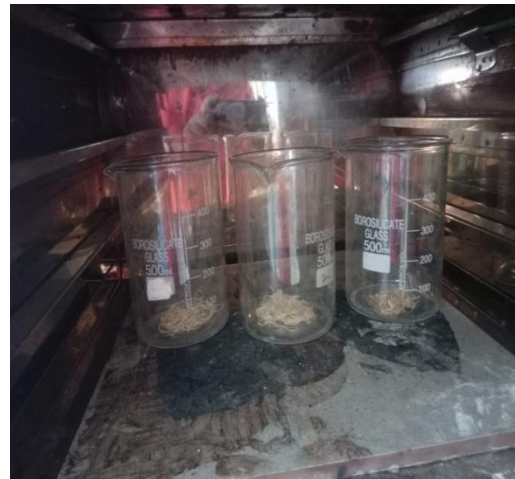
Fig 4.14 Treated fiber kept in oven
