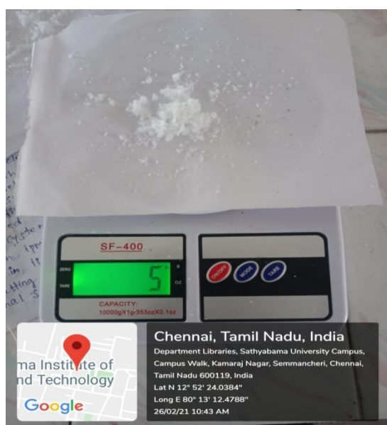
Fig 4.9 weighing 5 grams of NaOH
