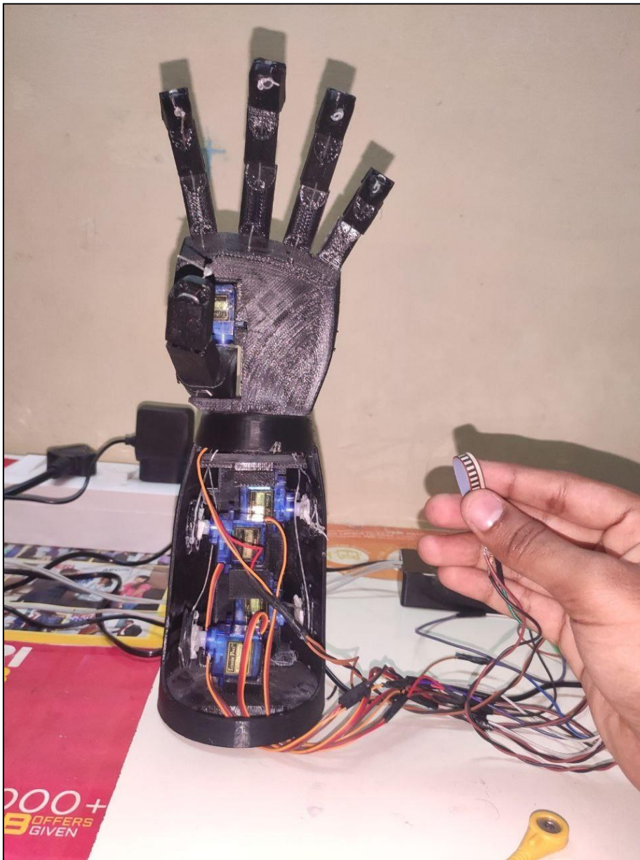
Figure 6.6: Single finger operation using the robotic hand.
