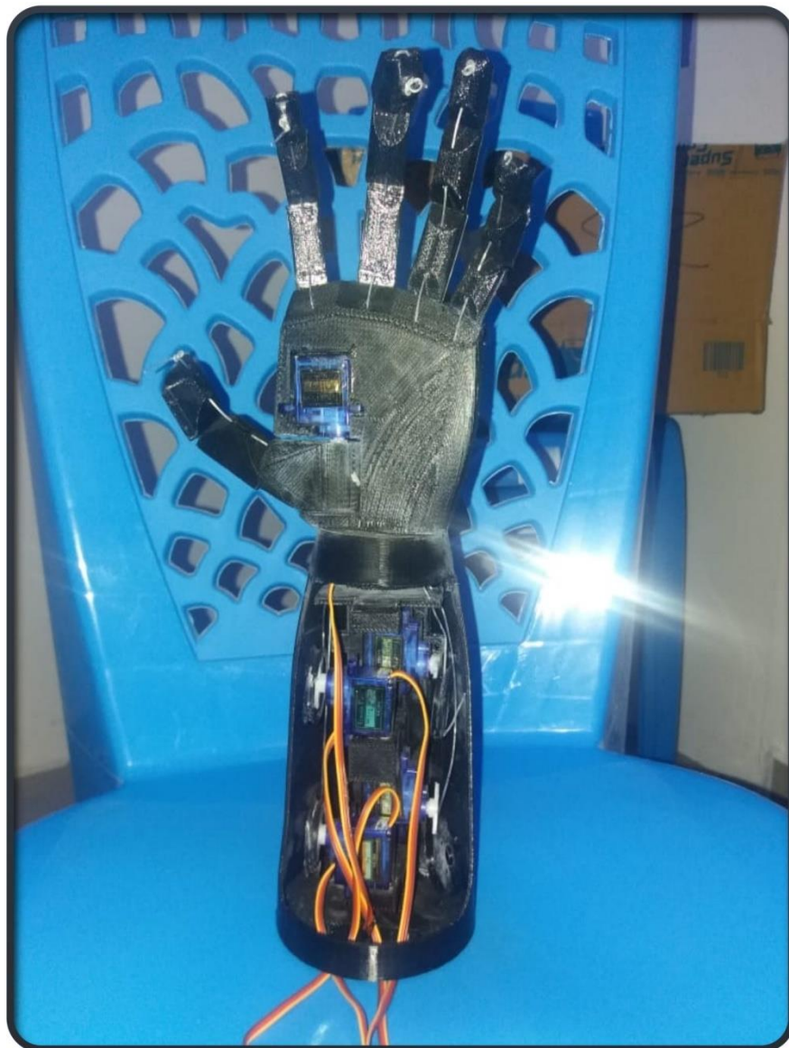
Figure 6.2: Acrylic hand servo motor integration
