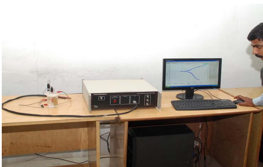
Fig. No. 17. Electrochemical properties test apparatus
