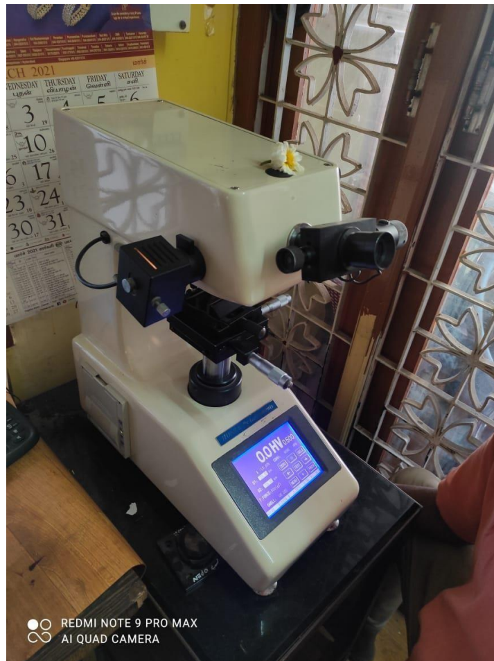
Fig.17 Hardness Test Setup
