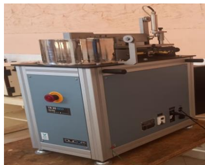
Figure 4.8: Pin on disc wear testing machine
