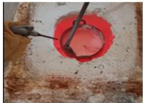
Fig 4.4: Skimming using Ar, SF 6 gas
