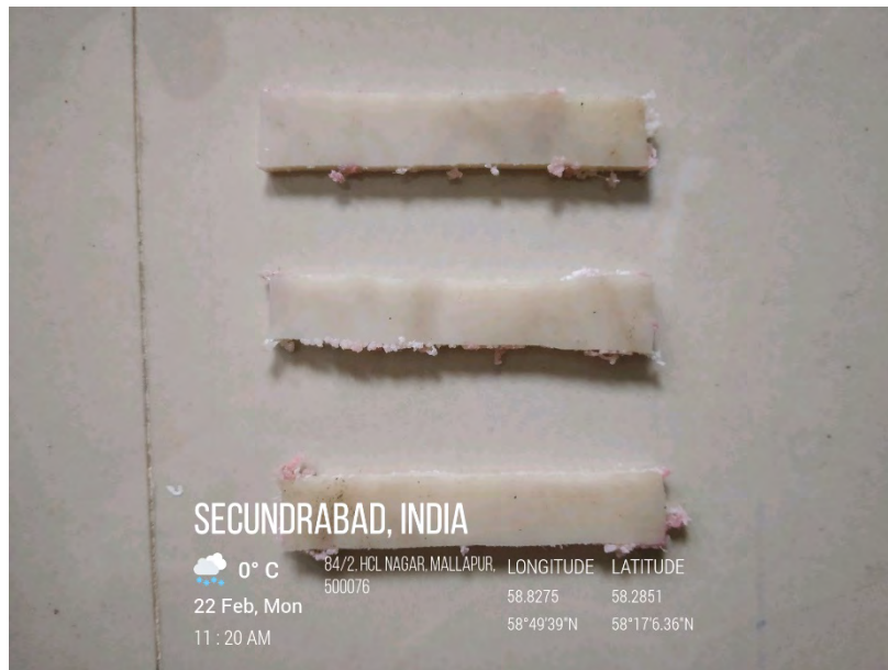
Fig:5.13 : Impact samples of pure PLA
