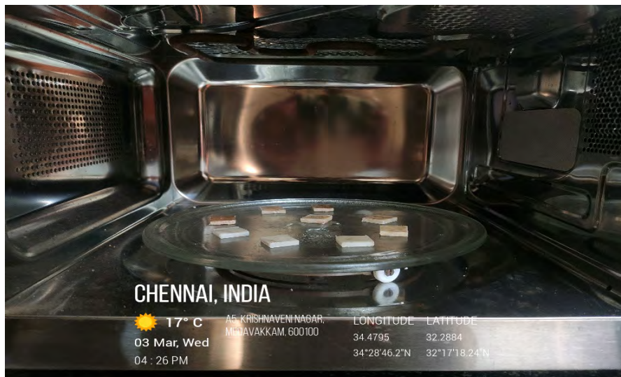
Fig:4.23 : Heating of water absorption samples
