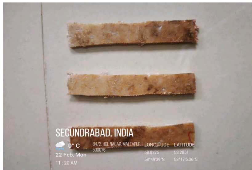
Fig:5.14 : Impact samples of PLA + untreated CQ fiber composite
