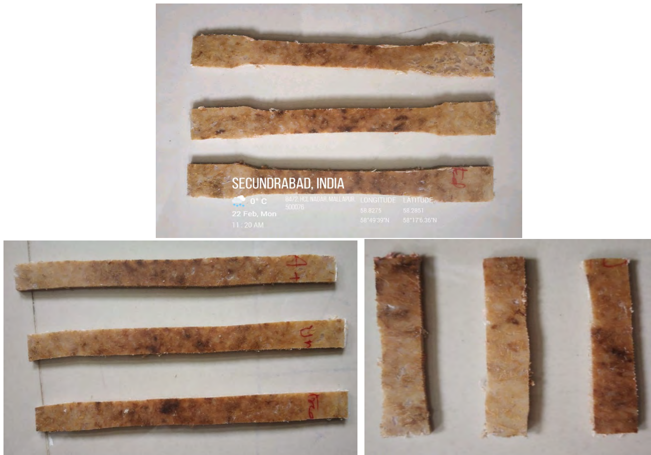
Fig:4.15 : Tensile, flexural and impact samples of untreated CQ fiber composite
