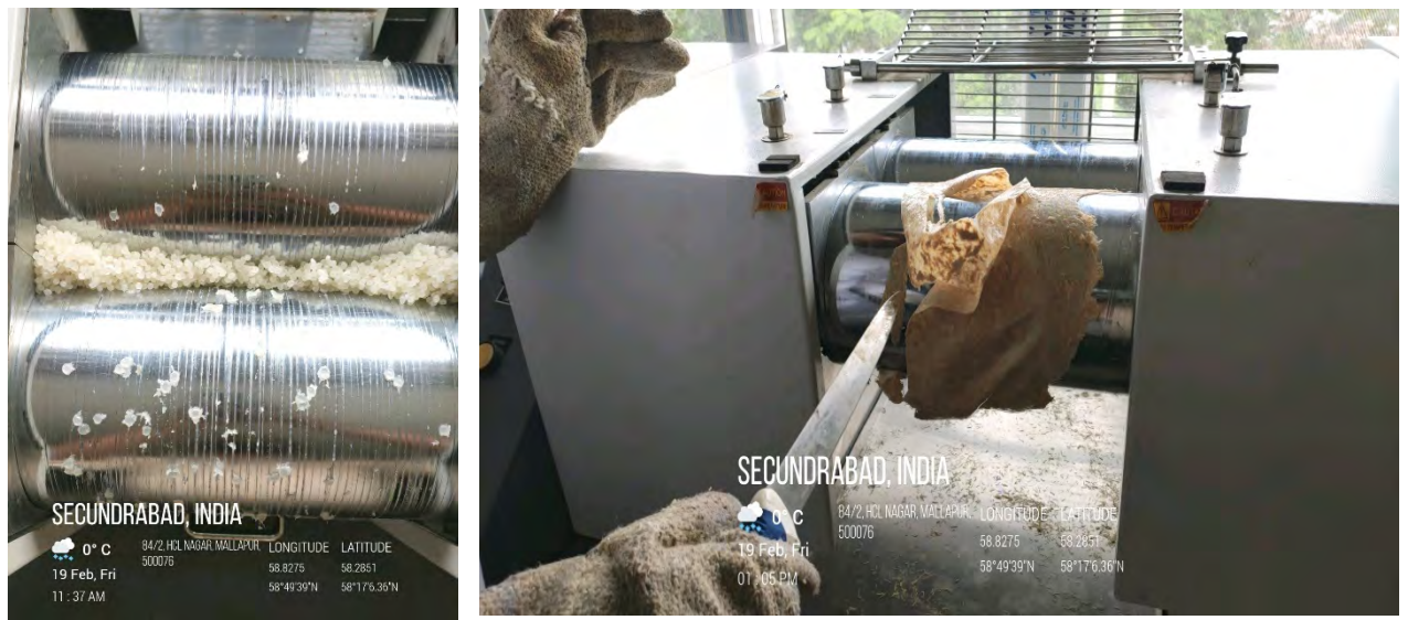
Fig:4.6 : Preparation of PLA and CQ fiber sheets using two roller machine
