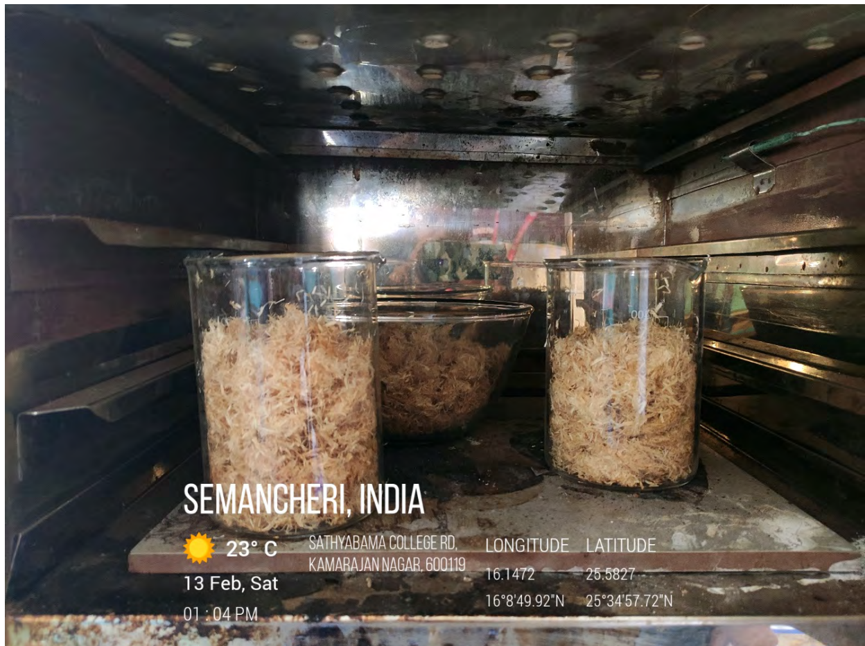
Fig:4.5 : Removing the moisture present in the fiber using hot chamber
