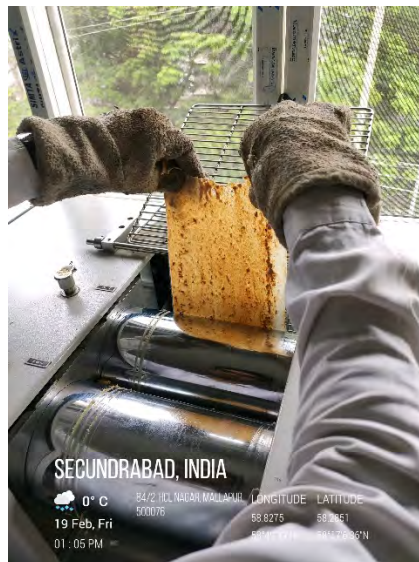
Fig:4.7 : Extraction of PLA and CQ fiber into sheet form
