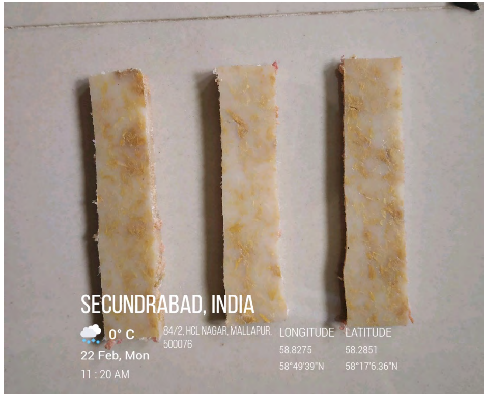
Fig:5.15 : Impact samples of PLA + treated CQ fiber composite
