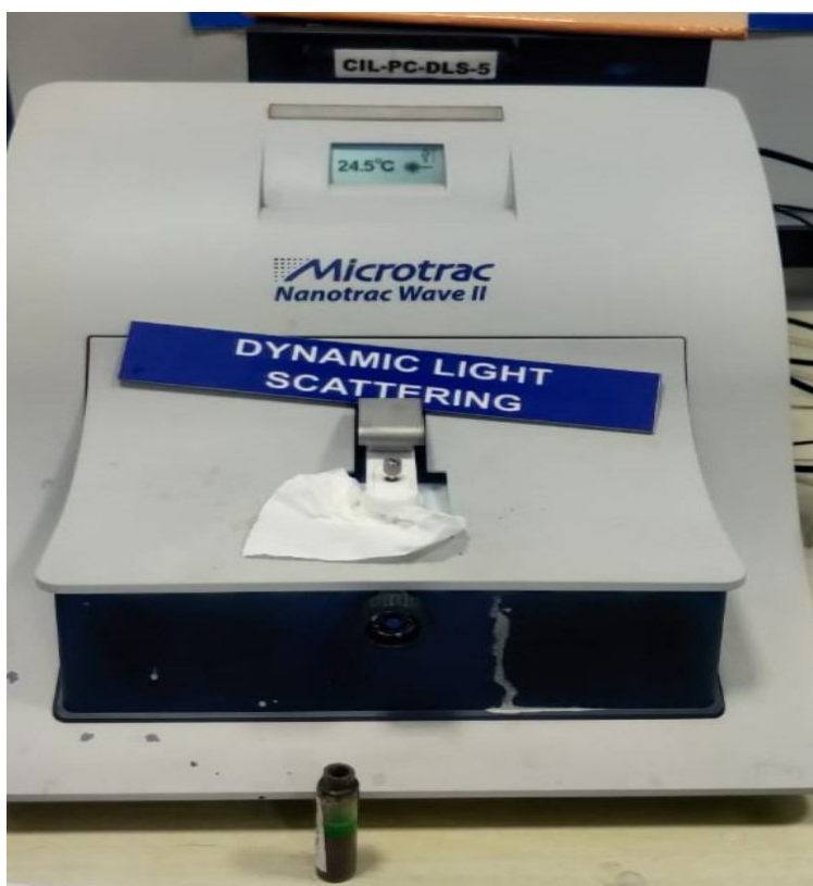
Fig 5.4: Dynamic light scattering machine
