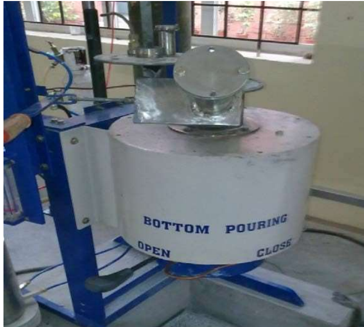
Figure 4.2 Stir Casting Furnace with Bottom Pouring
