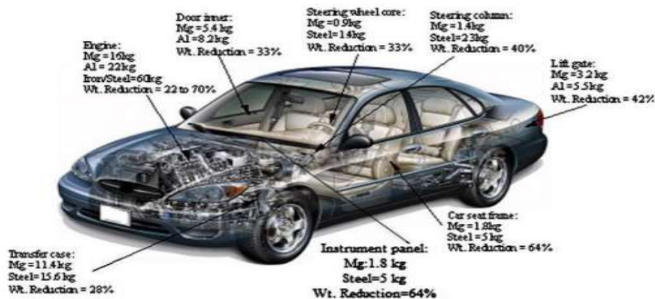
Figure 1.2 Some Automotive Components Made of Mg Alloy and Obtained Weight Reduction
