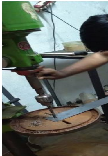
FIG 4.22 DRILLING CENTRE HOLE USING DRILL BIT @12.5 MM
