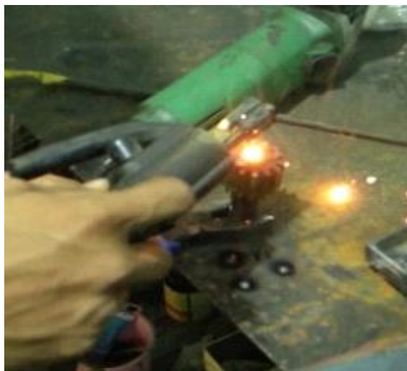
FIG 4.47 JOINING OF CYLINDRICAL SHAFT & PINION GEAR USING ARC WELDING
