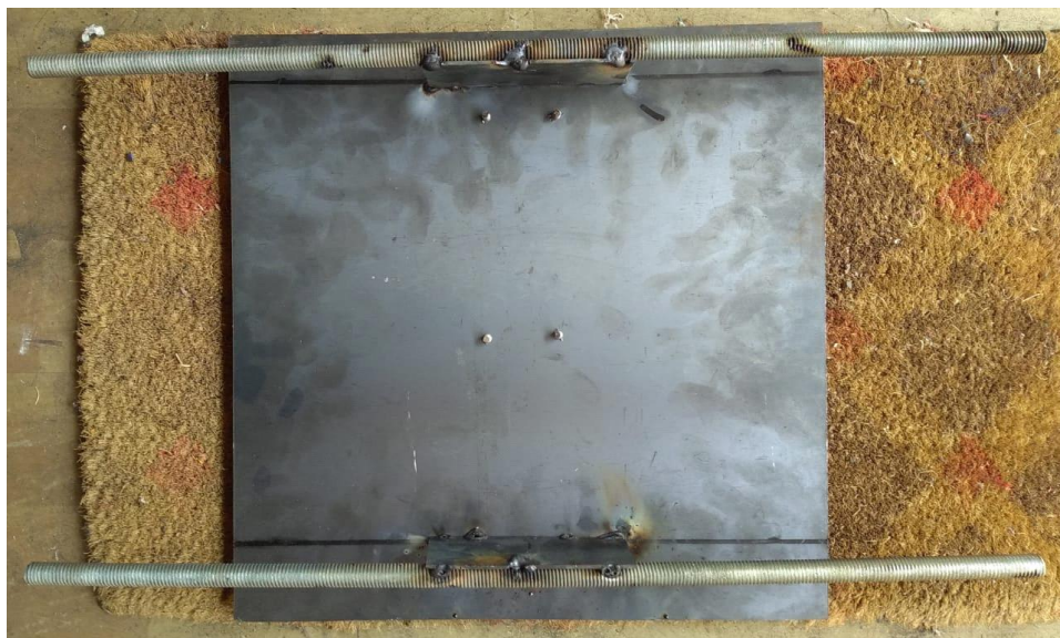
FIG 4.30 VIEW OF THREADED RODS AFTER WELDING TO MAIN FRAME
