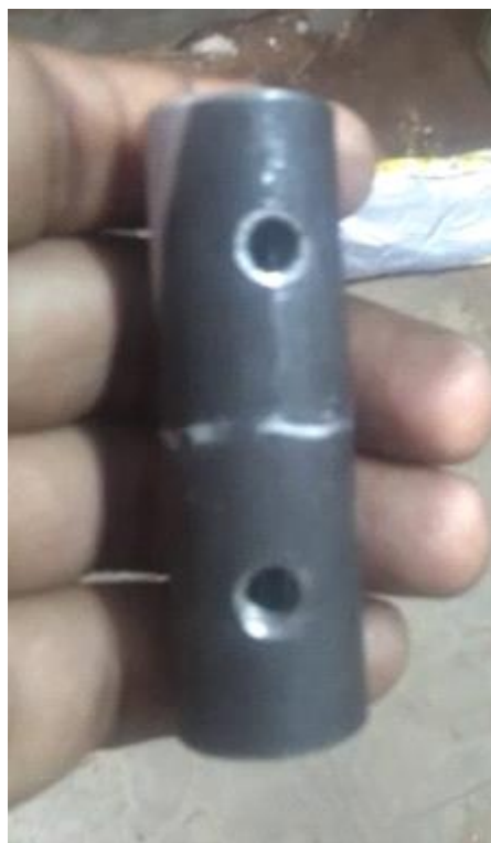
FIG 4.49 CYLINDRICAL SHAFT WITH THREADING WELDED TO ARM
