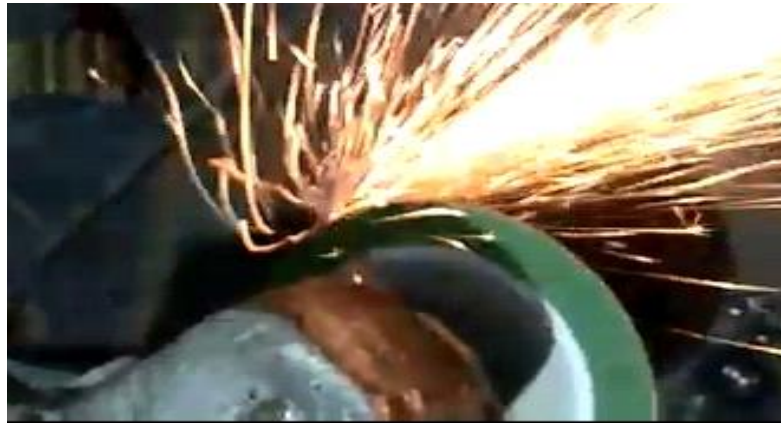
FIG 4.48 SURFACE GRINDING AFTER JOINING PROCESS
