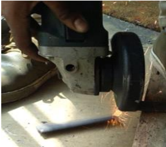
FIG 4.38 CUTTING OF ARM @ 115 MM
