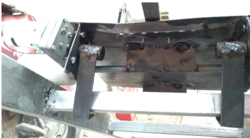
FIG 4.40 VIEW OF LOWER ARMS ON THE LADDER
