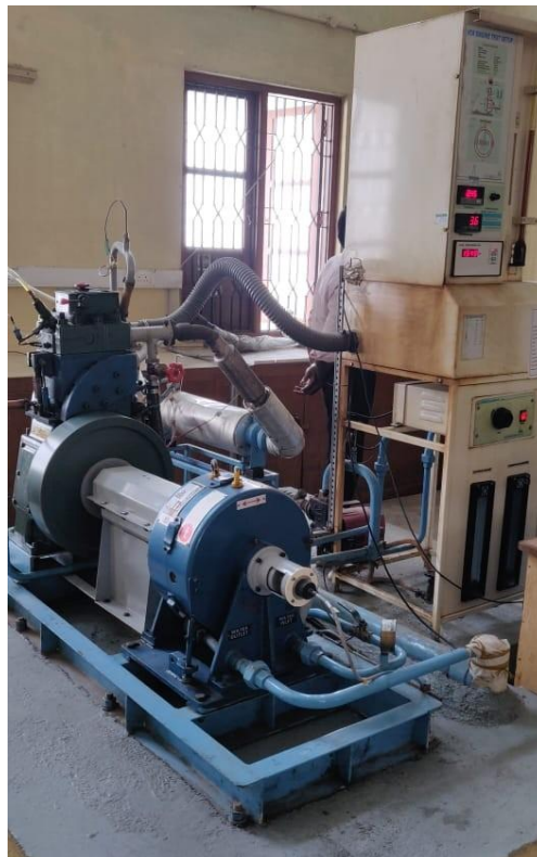
Fig: 4.3: The Layout of the Engine Test Bench
