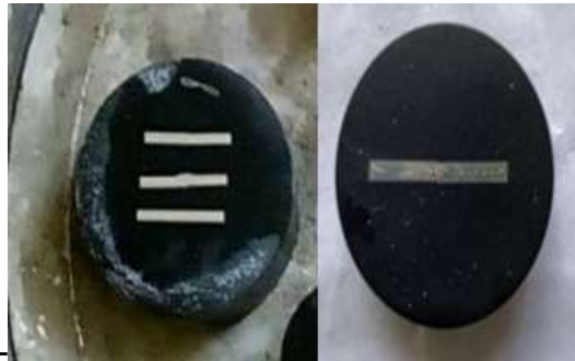
Fig: 4.18 Polished IRSM 41-97 specimens being dried water at room temperature
