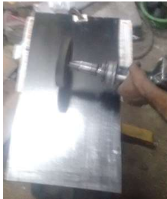
Fig: 4.4 Surface grading operation of IRSM 41-97 rail steel
