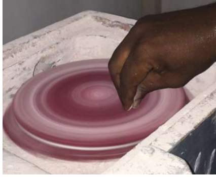
Fig: 4.17 IRSM 41-97specimens polished with alumina powder
