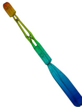
Fig 5.12: Displacement for after optimization for scissor rod
