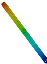
Fig 5.6: Displacement for before optimization for scissor rod
