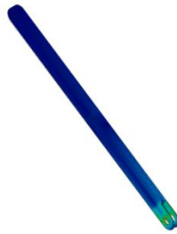
Fig 5.5 : Stress for before optimization for scissor rod
