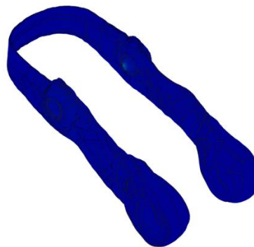
Figure 5.77: Stress for after optimization of Wishbone during Lateral torsional Force towards Right
