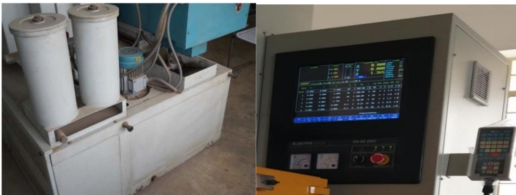
Fig: 4.3: Circulating pump and Control unit
