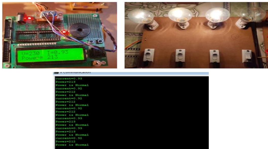
Fig. 5.5 : Output(4) 40+60+100W bulb is switched ON
