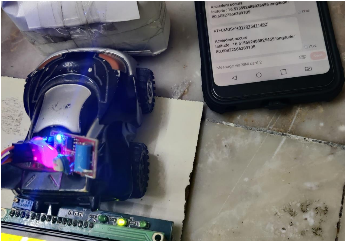
Fig: 5.3 Notification of Accident by vibration sensor
