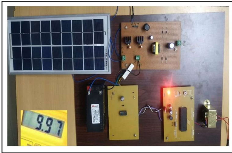
Fig5.10 Output Solar Voltage
