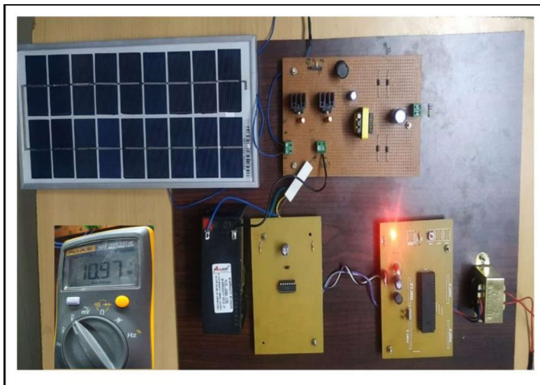
Fig5.11 Output Battery Voltage
