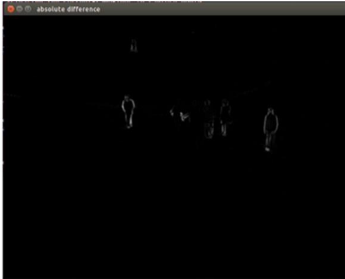
Fig.4.3 ABSOLUTE DIFFERENCE BETWEEN REFERENCE IMAGE AND CAPTURED IMAGE
