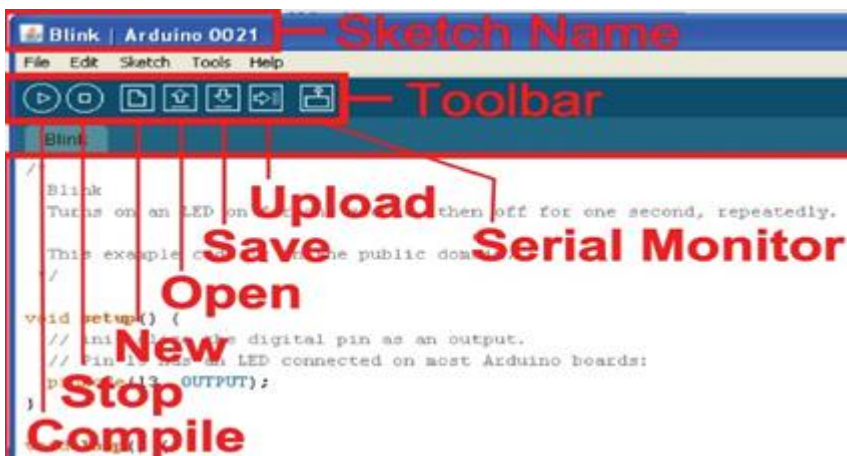
Fig 5.3.8: Upload the program to our board
