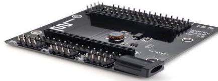
Fig 4.15 Node MCU Base Board
