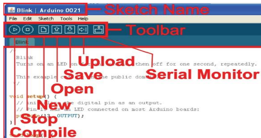
Fig 4.23: Upload the program to our board
