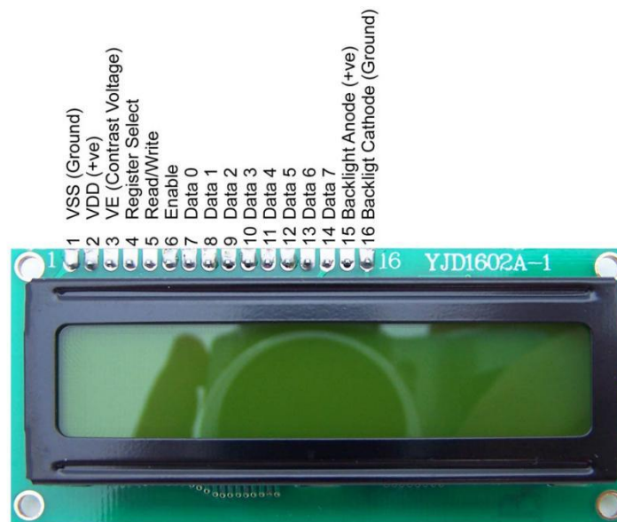
Fig 4.5 16x2 line Hitachi HD44780 display
