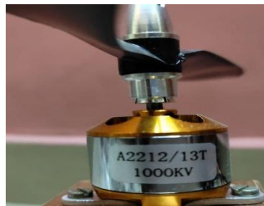
Fig 4.14 A2212/13T (BLDC) MOTOR
