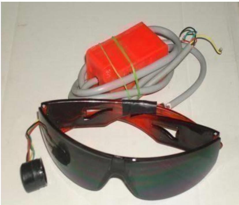
Fig.2.1.1. Connection of eye blink sensor with spectacles
