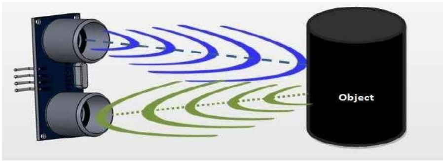
FIG: 4.11 ULTRASONIC SENSOR WORKING
