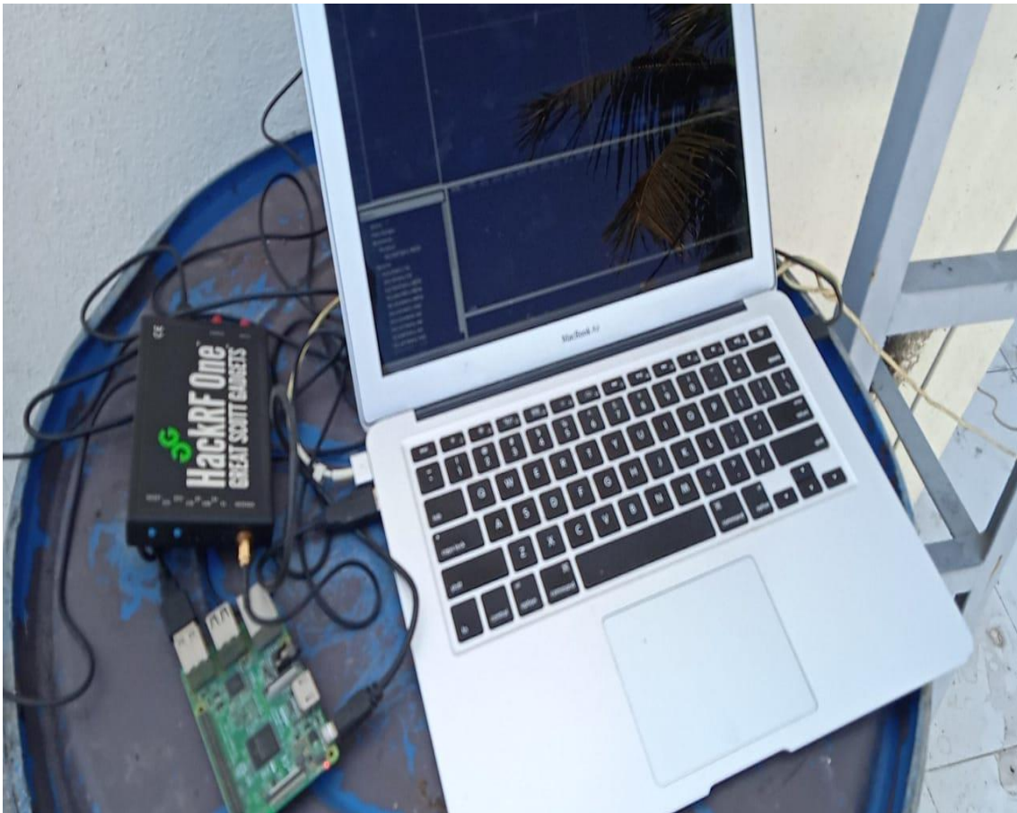
Fig: 4.1: Setup used for reception of satellite signals
