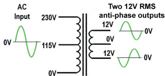
Fig 3.3 Step down Transformer
