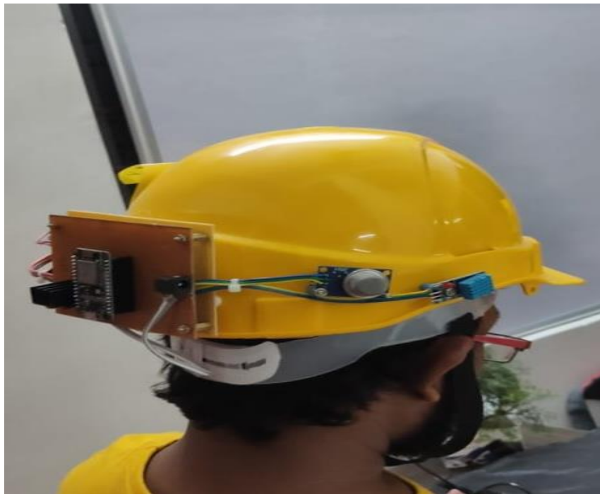
Fig.5.2. Smart Helmet with Sensors
