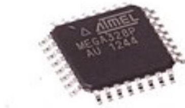
Fig.no 1.1 ATmega328P in 32-pin thin quad flat pack (TQFP-32)
