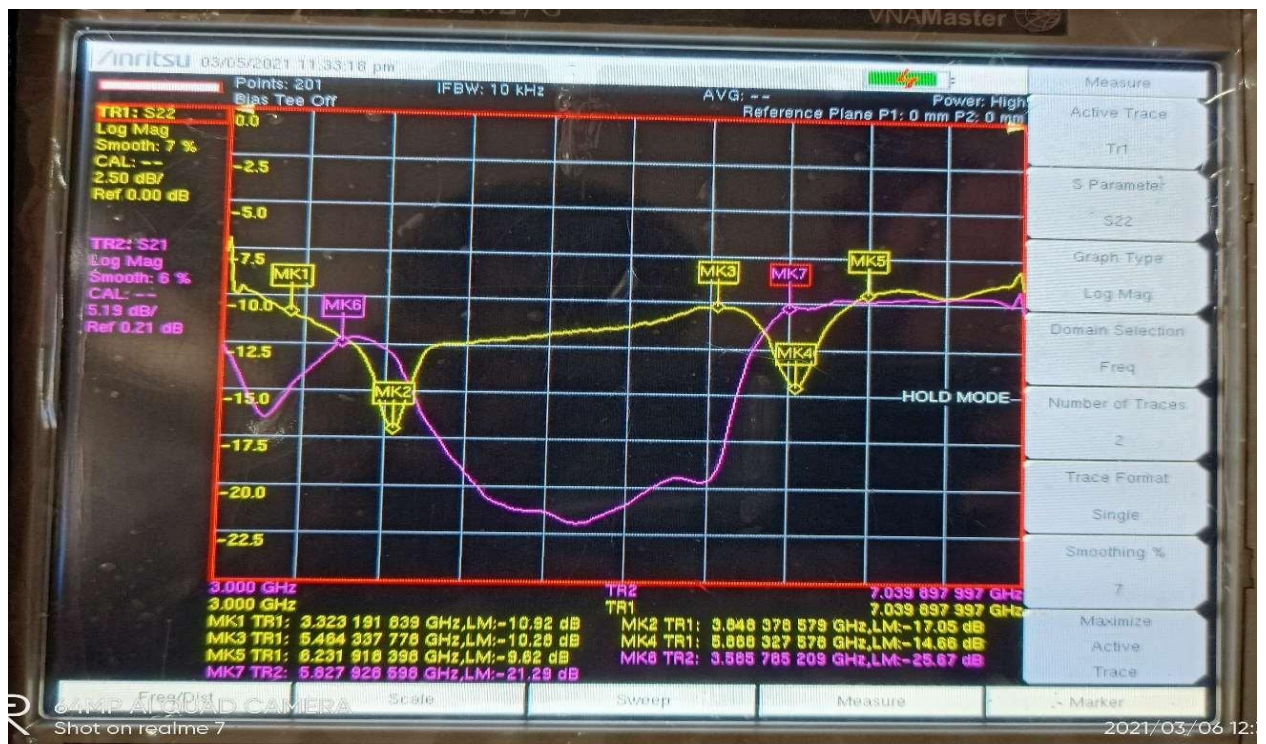
Fig 26 Notching and passing parameter at S22.
