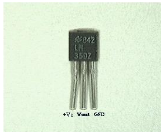
Fig 4.12: View of temperature sensor
