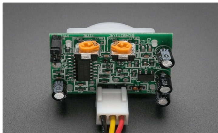
Fig 5.10 Changing Pulse Time and Timeout Length
