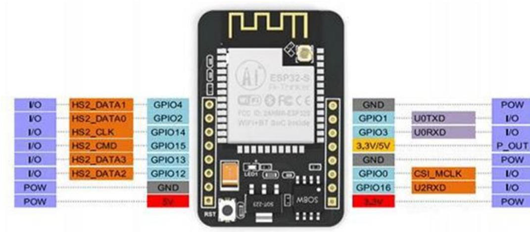
Fig 4.8- ESP32-CAM Pinout
