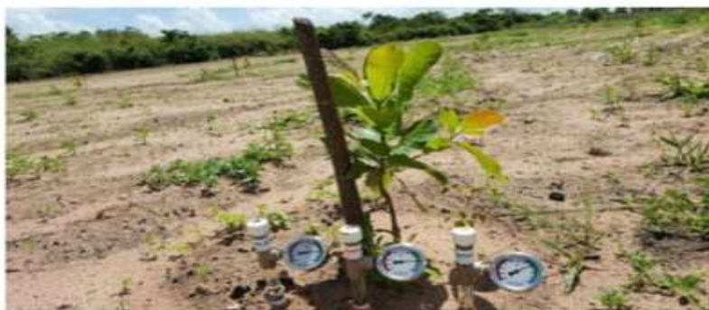
(a) Tensiometers at 15, 45, and 75 cm depths near a cashew bud.
