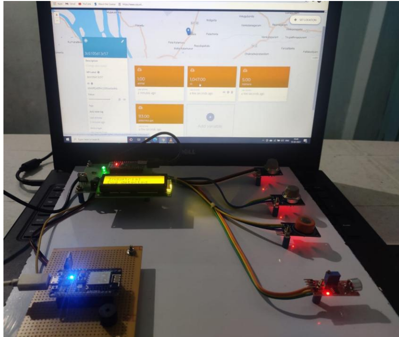
Fig :5.2 : CONNECTION TO SERVER
