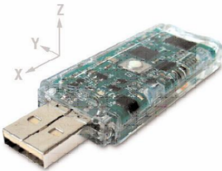
FIG. 7. The 3-axis USB sensor can be used as a design and evaluation tool when researching or launching a new design.
