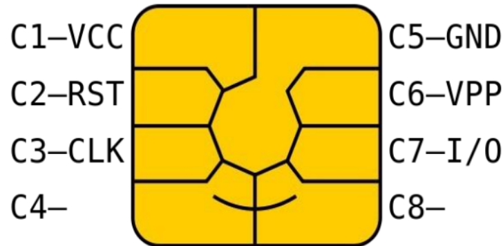
Figure 2.3: Standard pin-out of a simple Smart card chip according to ISO-7816.
