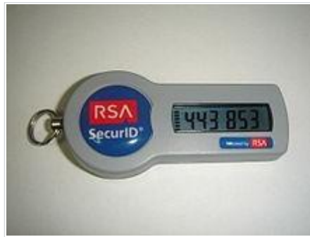
Figure 2.1: RSA SecurID token, an example of a disconnected token generator
