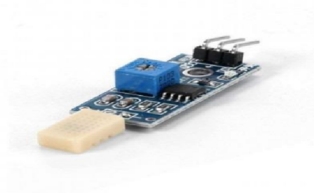
Fig : 4.5: Humidity sensor
