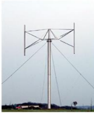
Figure 3.5. Giromill type wind turbine
