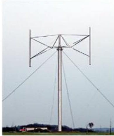
Figure 3.5. Giromill type wind turbine
