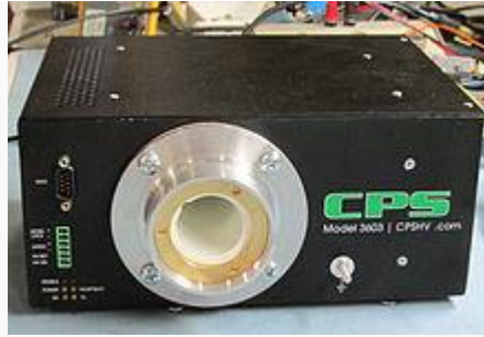
Fig:4.11.8 A High Voltage power supply
