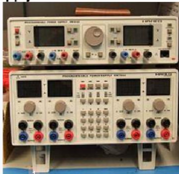
Fig:4.11.7 Programmable power supplies
