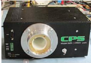
Fig:4.11.8 A High Voltage power supply
