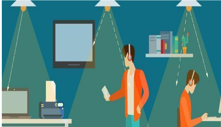
Fig 3.5 basic concept of Li-Fi
