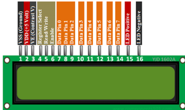
Figure 4.1.2 c LCD PIN DESCRIPTION
