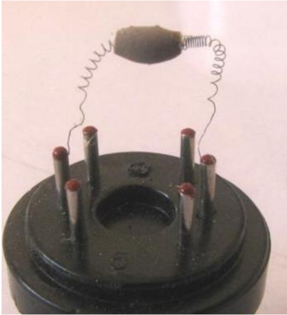
Fig 4.8.5:Nickel-chromium detecting component
